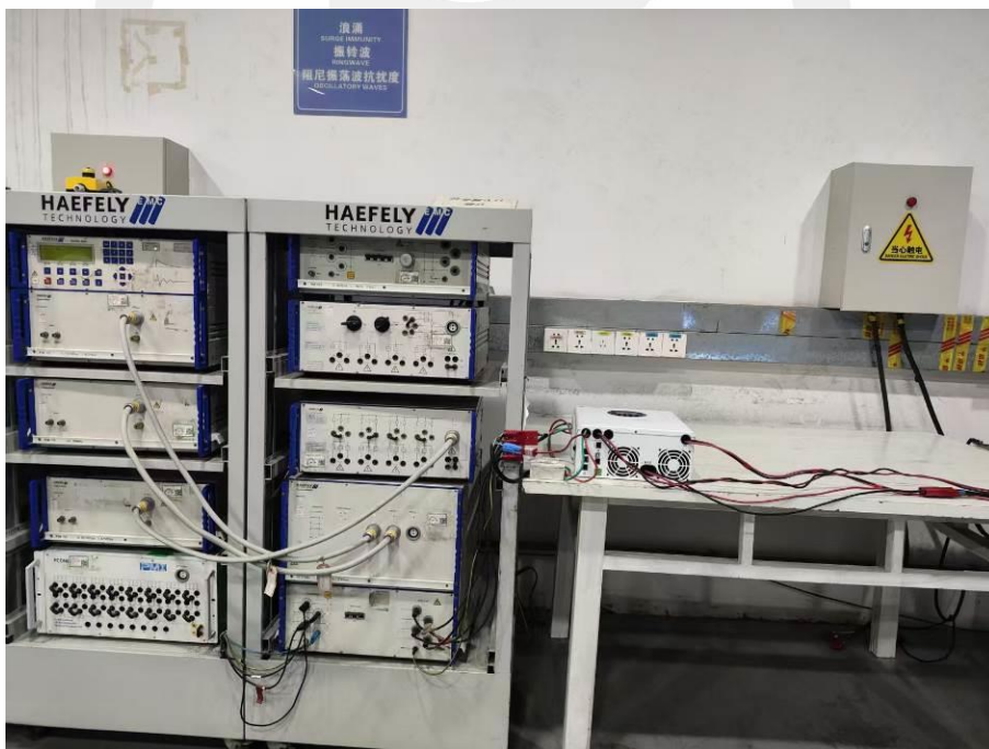
16.7.Photo of Surge Test
