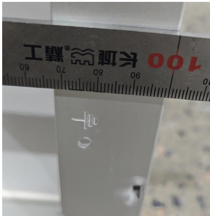
Fig. 8: detail view of equipotential bonding hole and symbol
