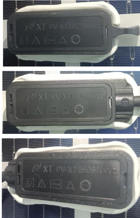
Fig. 5: detail view of closed junction box
