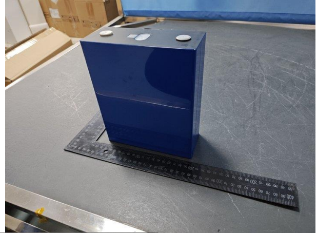
内部电芯 / Component Cell (LFP71173207/314Ah 3,2V 314Ah 1004,8Wh)
