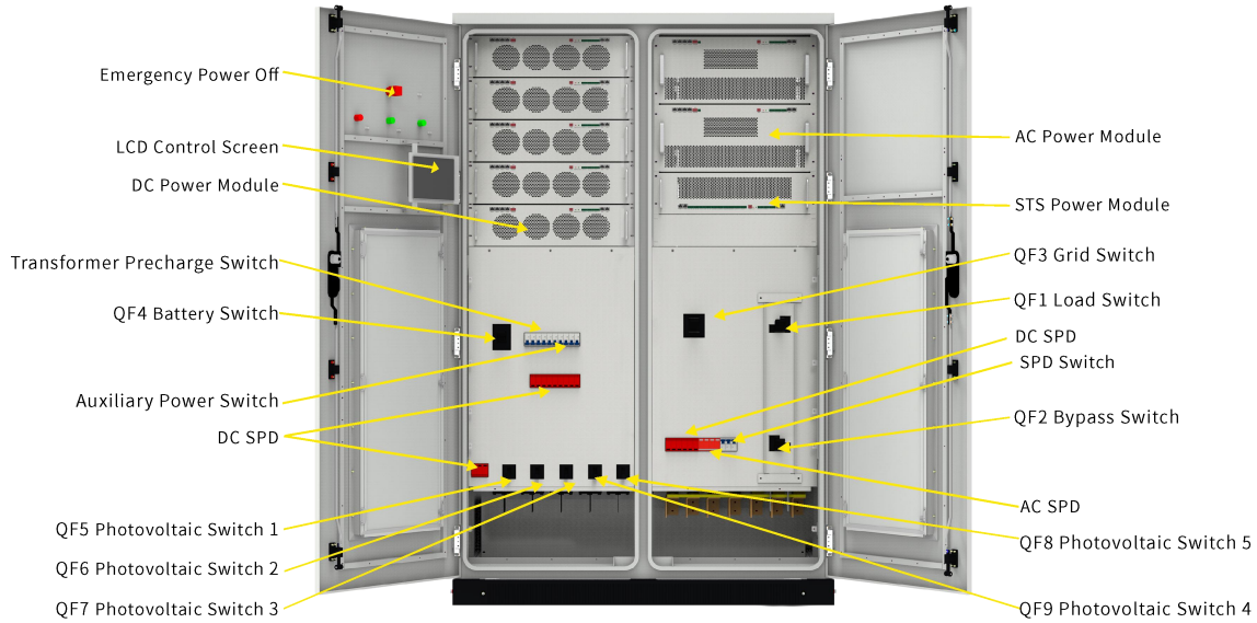
Figure 2-3 Cabinet internal structure diagram
