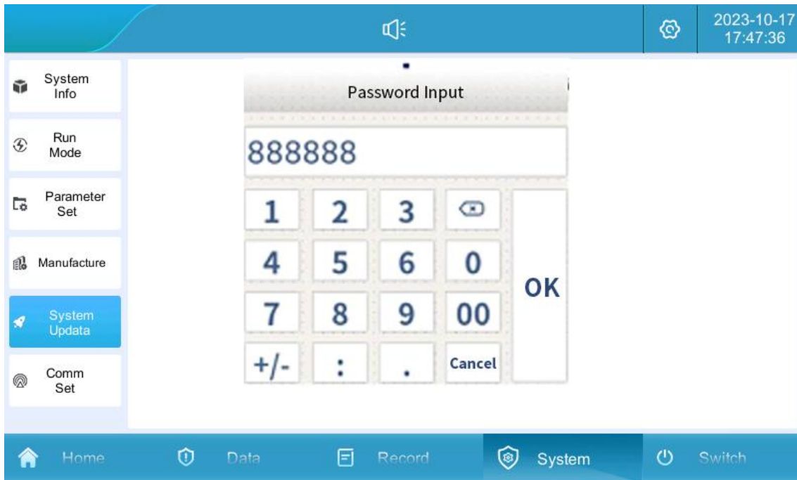
Figure 5-20 Upgrade Software Password Verification
