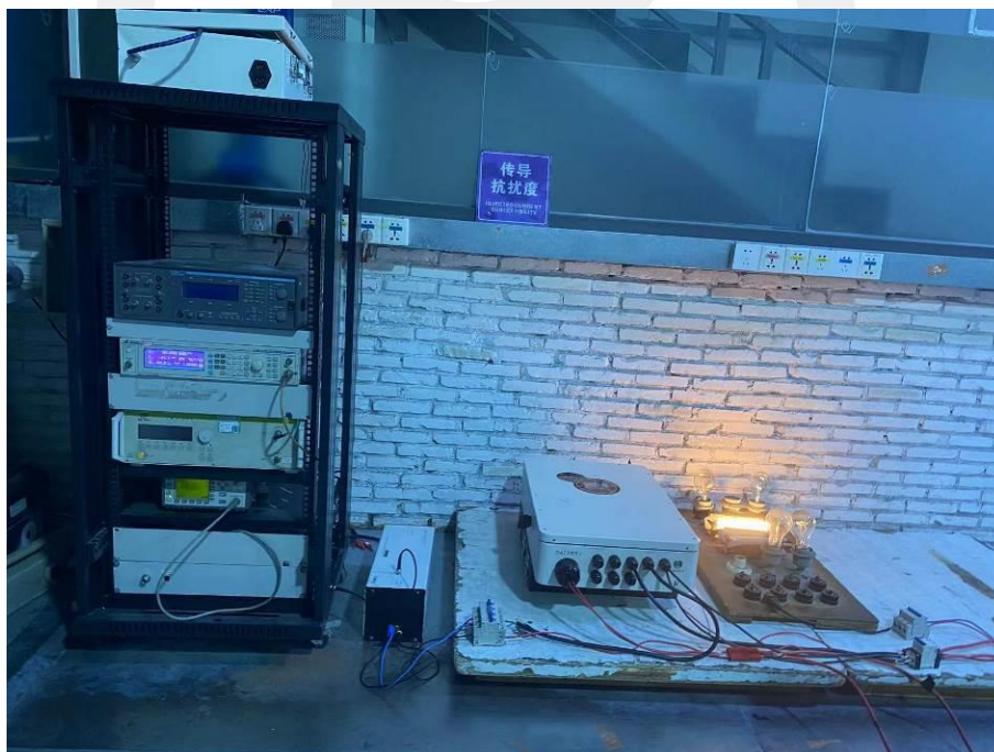
16.8.Photo of Injected Currents Susceptibility Test
